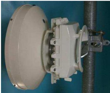
Separated ODU and parabolic antenna
