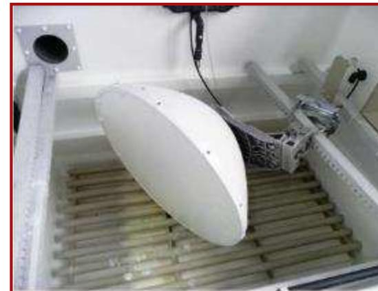
**Tested against humidity and corrosion**
