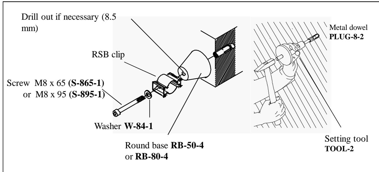
In case of fire the resistant part of the fixing will hold the cable in position and enables the cable to keep in operation as long as the cable itself allows. It also prevents the cable from detaching from the wall that might block any escape route.
