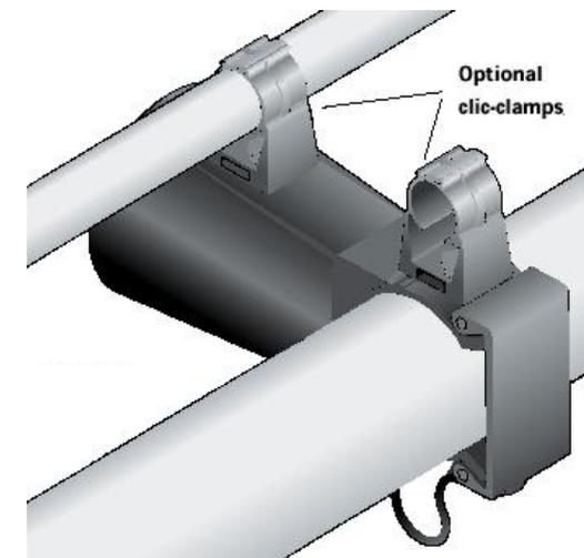
Optional up to 4 additional clic-clamps could be mounted e.g. optic backbone cables. Suitable types are [CC-12-2](#), [CC-58-2](#) & [CC-78-2](#)
